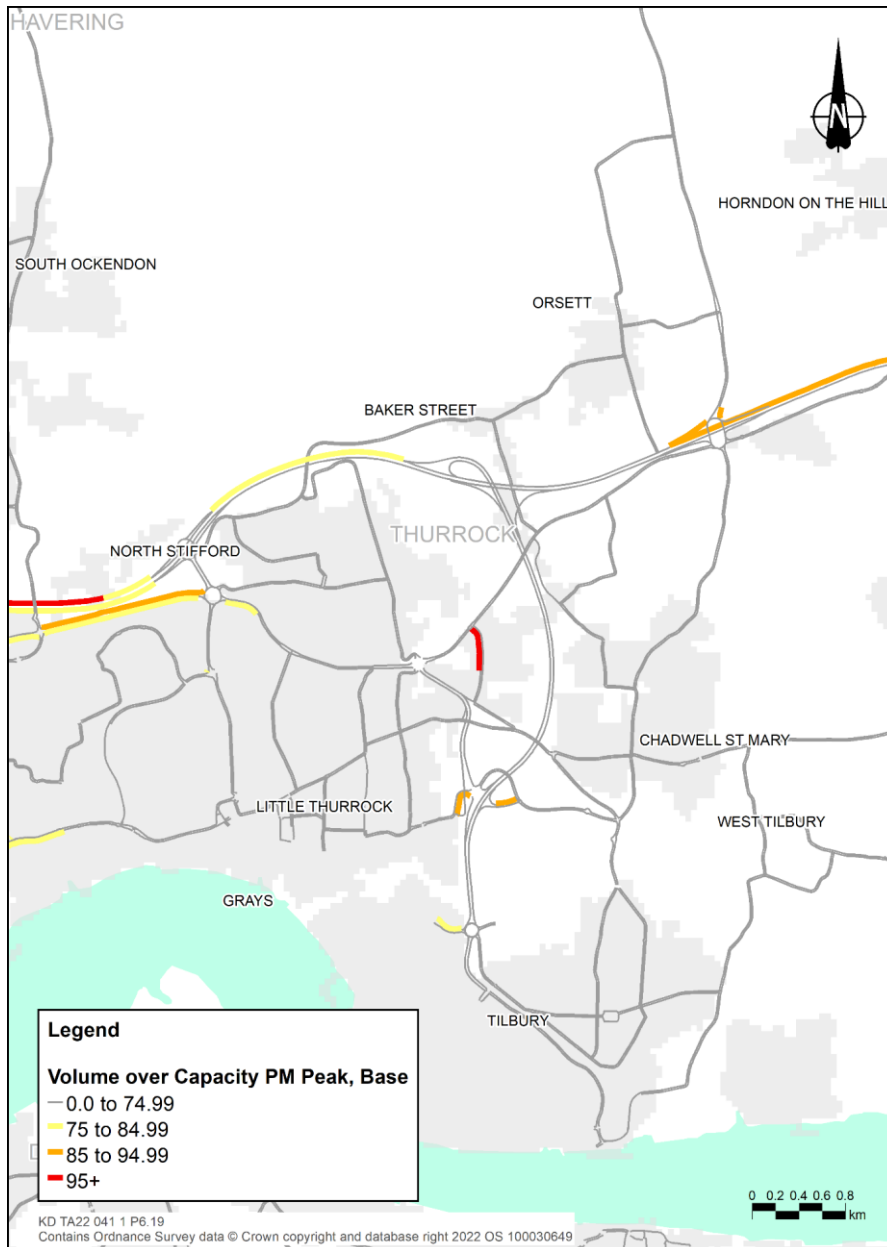
Plate 6.19 Volume to capacity 2016 PM peak (17:00-18:00) at the A13/A1089/A122 Lower Thames Crossing junction
