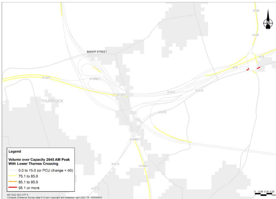
Plate 7.5 Volume to capacity at the A13/A1089/A122 Lower Thames Crossing junction – AM peak 2045
